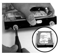
4. Install 4 white Anti-Shock Mounts w/10mm screw into both sides of the hard drive. Do not tighten the screws yet.
